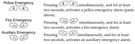
The resulting annunciation, along with other system sounds is configurable. If your system has been programmed to do so, it will communicate any or all of these alarms to the station monitoring your installation. System programming also determines whether these emergency alarms are audible and/or capable of being communicated to the monitoring station.
